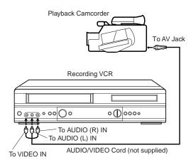
For duplicating a previously recorded tape from a camcorder, follow the camcorder manufacturer's instructions. A typical camcorder dubbing hookup is shown above.
